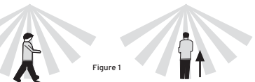
Walking tangential to the sensor (normal detection range) Walking directly to the sensor (lower detection range)
